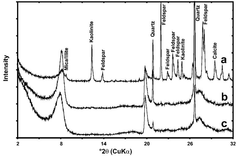
Figure 16. XRD patterns of size-fractions of ISMt-1 illite-smectite separated using deionized water only. Fraction A: gravity settled after 5 min for an additional 60 min (5–18  $\mu\text{m}$ ); Fraction B: gravity settled for an additional 64 h (0.7–5  $\mu\text{m}$ ); and Fraction C: centrifuged using a Sorvall GSA head at 5000 RPM for 5 min (0.25–0.7  $\mu\text{m}$ ).
