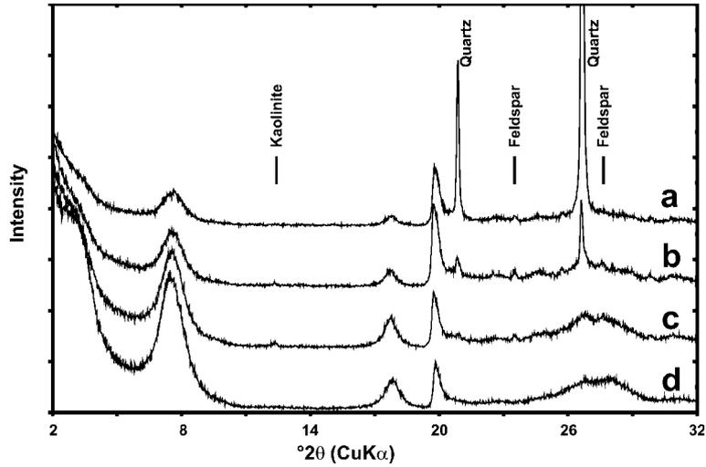
Figure 15. XRD patterns of size-fractions of ISCz-1 illite-smectite separated using deionized water only. Fraction A: gravity settled after 5 min for an additional 60 min (5–18  $\mu\text{m}$ ); Fraction B: gravity settled for an additional 16 h (1.5–5  $\mu\text{m}$ ); Fraction C: centrifuged using a Sorvall GSA head at 5000 RPM for 5 min (0.25–1.5  $\mu\text{m}$ ); and Fraction D: centrifuged using a Sorvall GSA head at 8000 RPM for 40 min (0.1–0.25  $\mu\text{m}$ ).
