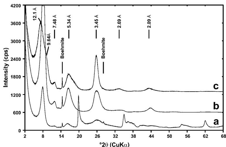
Figure 7. XRD patterns of the 'processed'  $<2 \mu\text{m}$  size-fraction of Syn-1 mica-montmorillonite: (a) random (collected at 11% RH;  $001 = 11.2 \text{ \AA}$ ); (b) oriented (collected at 5% RH;  $001 = 10.9 \text{ \AA}$ ); and (c) oriented and glycolated ( $001 = 12.1 \text{ \AA}$ ).
