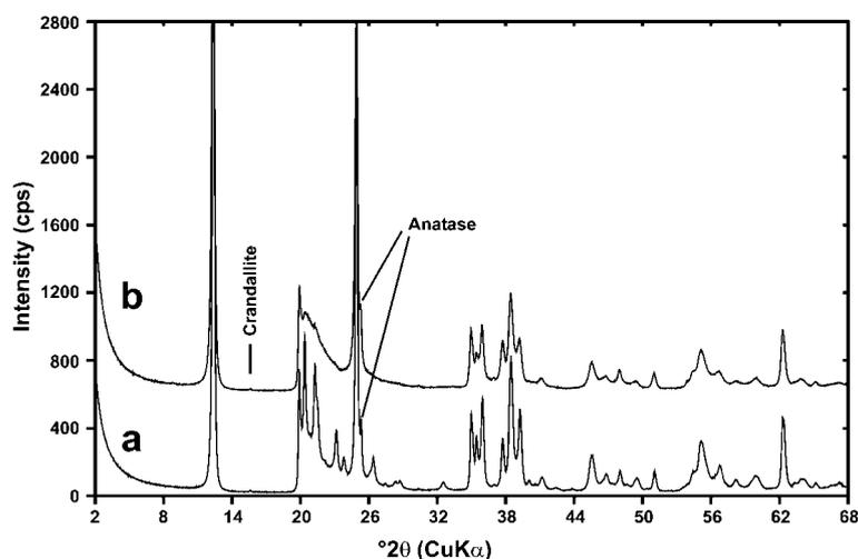
Figure 1. XRD patterns of the ‘processed’ <2 μm size-fraction of (a) KGa-1b and (b) KGa-2.
