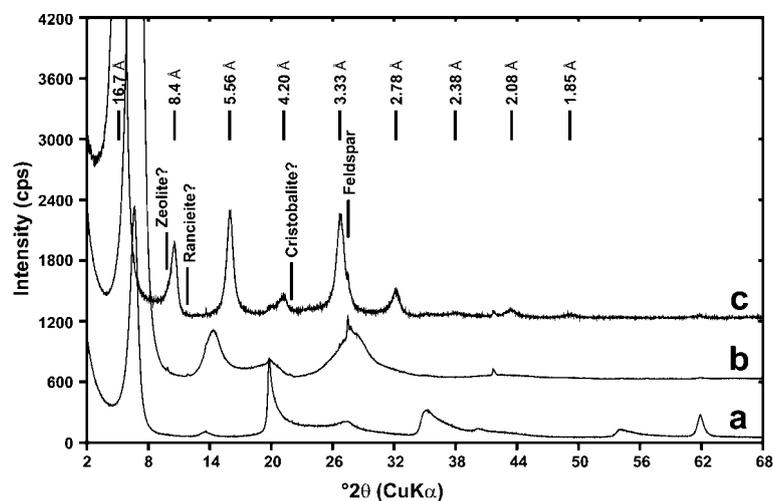
Figure 3. XRD patterns of the 'processed'  $<2 \mu\text{m}$  size-fraction of SAz-1 smectite: (a) random (collected at 6% RH;  $001 = 13.3 \text{ \AA}$ ); (b) oriented (collected at 3% RH;  $001 = 13.0 \text{ \AA}$ ); and (c) oriented and glycolated ( $001 = 16.7 \text{ \AA}$ ).
