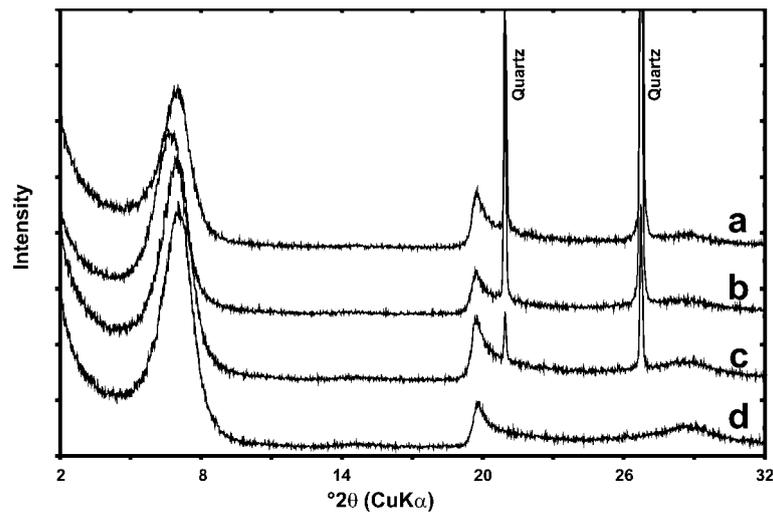
Figure 18. XRD patterns of size-fractions of SWa-1 ferruginous smectite separated using deionized water only. Fraction A: gravity settled after 5 min for an additional 60 min (5–18  $\mu\text{m}$ ); Fraction B: gravity settled for an additional 64 h (0.7–5  $\mu\text{m}$ ); Fraction C: centrifuged using a Sorvall GSA head at 5000 RPM for 5 min (0.25–0.7  $\mu\text{m}$ ); and Fraction D: centrifuged using a Sorvall GSA head at 8000 RPM for 60 min (0.1–0.25  $\mu\text{m}$ ).
