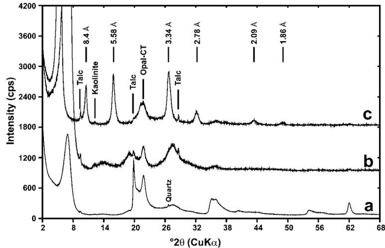
Figure 4. XRD patterns of the 'processed'  $<2 \mu\text{m}$  size-fraction of STx-1 smectite: (a) random (collected at 24% RH;  $001 = 12.8 \text{ \AA}$ ); (b) oriented (collected at 3% RH;  $001 = 12.7 \text{ \AA}$ ); (c) oriented and glycolated ( $001 = 16.8 \text{ \AA}$ ).
