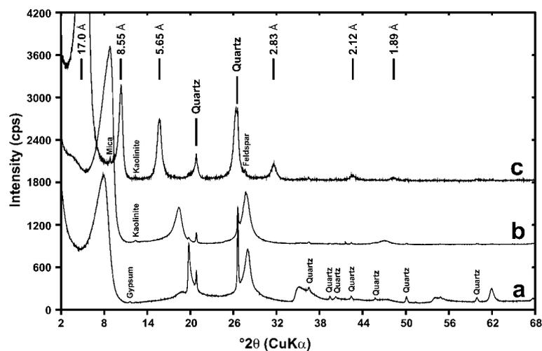
Figure 5. XRD patterns of the 'processed'  $<2 \mu\text{m}$  size-fraction of SWy-2 smectite: (a) random (collected at 9% RH;  $001 = 11.2 \text{ \AA}$ ); (b) oriented (collected at 3% RH;  $001 = 10.1 \text{ \AA}$ ); and (c) oriented and glycolated ( $001 = 17.0 \text{ \AA}$ ).
