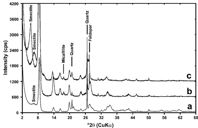
Figure 2. XRD patterns of the 'processed'  $<2 \mu\text{m}$  size-fraction of PFI-1 palygorskite: (a) random (collected at 24% RH;  $001_{\text{smectite}} = 13.8 \text{ \AA}$ ,  $110_{\text{palygorskite}} = 10.5 \text{ \AA}$ ); (b) oriented (collected at 5% RH;  $001_{\text{smectite}} = 13.5 \text{ \AA}$ ,  $110_{\text{palygorskite}} = 10.5 \text{ \AA}$ ); and (c) oriented and glycolated ( $001_{\text{smectite}} = 16.9 \text{ \AA}$ ,  $110_{\text{palygorskite}} = 10.7 \text{ \AA}$ ).
