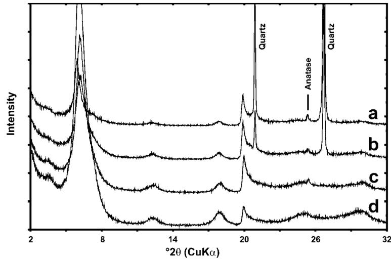
Figure 17. XRD patterns of size-fractions of SBCa-1 beidellite separated using deionized water only. Fraction A: gravity settled after 5 min for an additional 60 min (5–18  $\mu\text{m}$ ); Fraction B: gravity settled for an additional 16 h (1.5–5  $\mu\text{m}$ ); Fraction C: centrifuged using a Sorvall GSA head at 5000 RPM for 5 min (0.25–1.5  $\mu\text{m}$ ); and Fraction D: centrifuged using a Sorvall GSA head at 8000 RPM for 40 min (0.1–0.25  $\mu\text{m}$ ).
