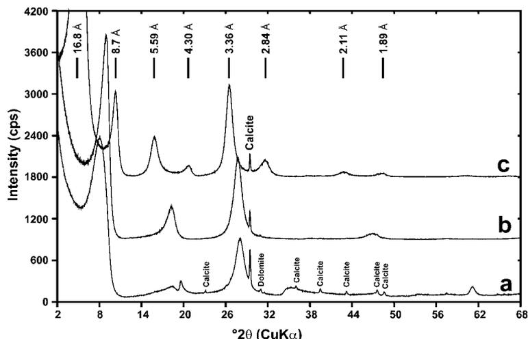
Figure 6. XRD patterns of the 'processed'  $<2 \mu\text{m}$  size-fraction of SHCa-1 hectorite: (a) random (collected at 6% RH;  $001 = 11.0 \text{ \AA}$ ); (b) oriented (collected at 5% RH;  $001 = 9.9 \text{ \AA}$ ); and (c) oriented and glycolated ( $001 = 16.8 \text{ \AA}$ ).
