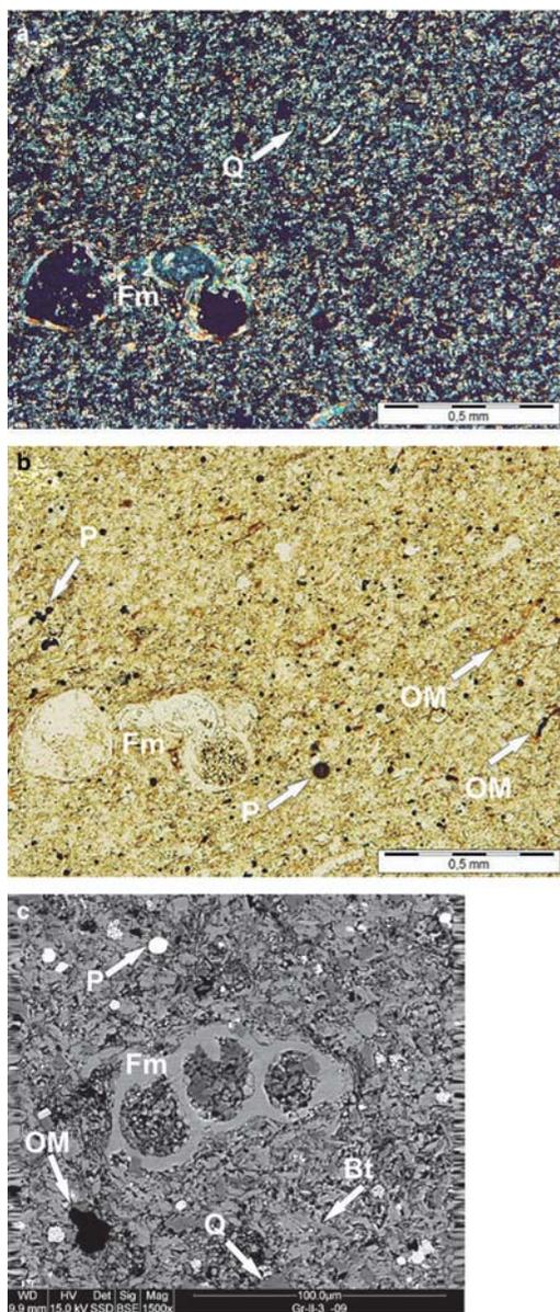
**Figure 2.** Microfabric of the Grybów Marls (sample Gr-II-3). Individual foram test (Fm), silt-size quartz grains (Q), biotite (Bt), pyrite framboids (P), and organic matter (OM), which are disseminated in the background. Thin-section micrograph (a – crossed polars; b – plane polarized light). c – coccolith fragments (white) and clay in the background captured in a FESEM/BSE image.
