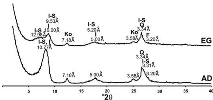
**Figure 1.** Representative XRD patterns of the fine clay fraction ( $<0.2 \mu\text{m}$ ) isolated from the Grybów Marl sample (G-II-3). AD – air-dried; EG – ethylene glycol solvated; I-S – illite-smectite, I – illite, Ko – kaolinite, Q – quartz.
