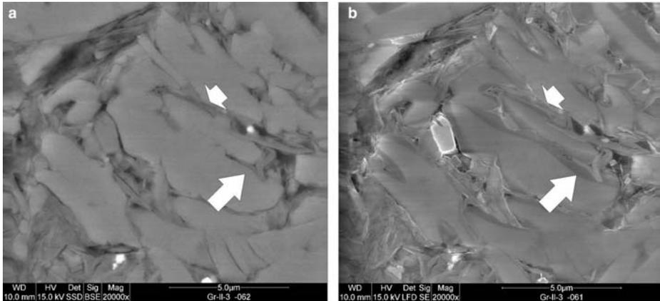
**Figure 3.** Interstices between coccolith shields partially cemented by pore-lining clay which postdate the overgrowth cement (longer arrows). Note the lamellar clay aggregates squeezed between overgrown coccoliths (shorter arrows). Grybów Marls, sample Gr-II-3: (a) FESEM/BSE and (b) CCI images.
