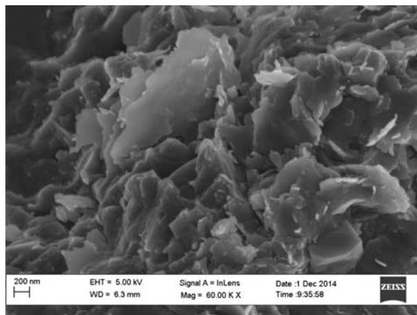
*Figure 3.* SEM image of the Hontomin shale sample.
