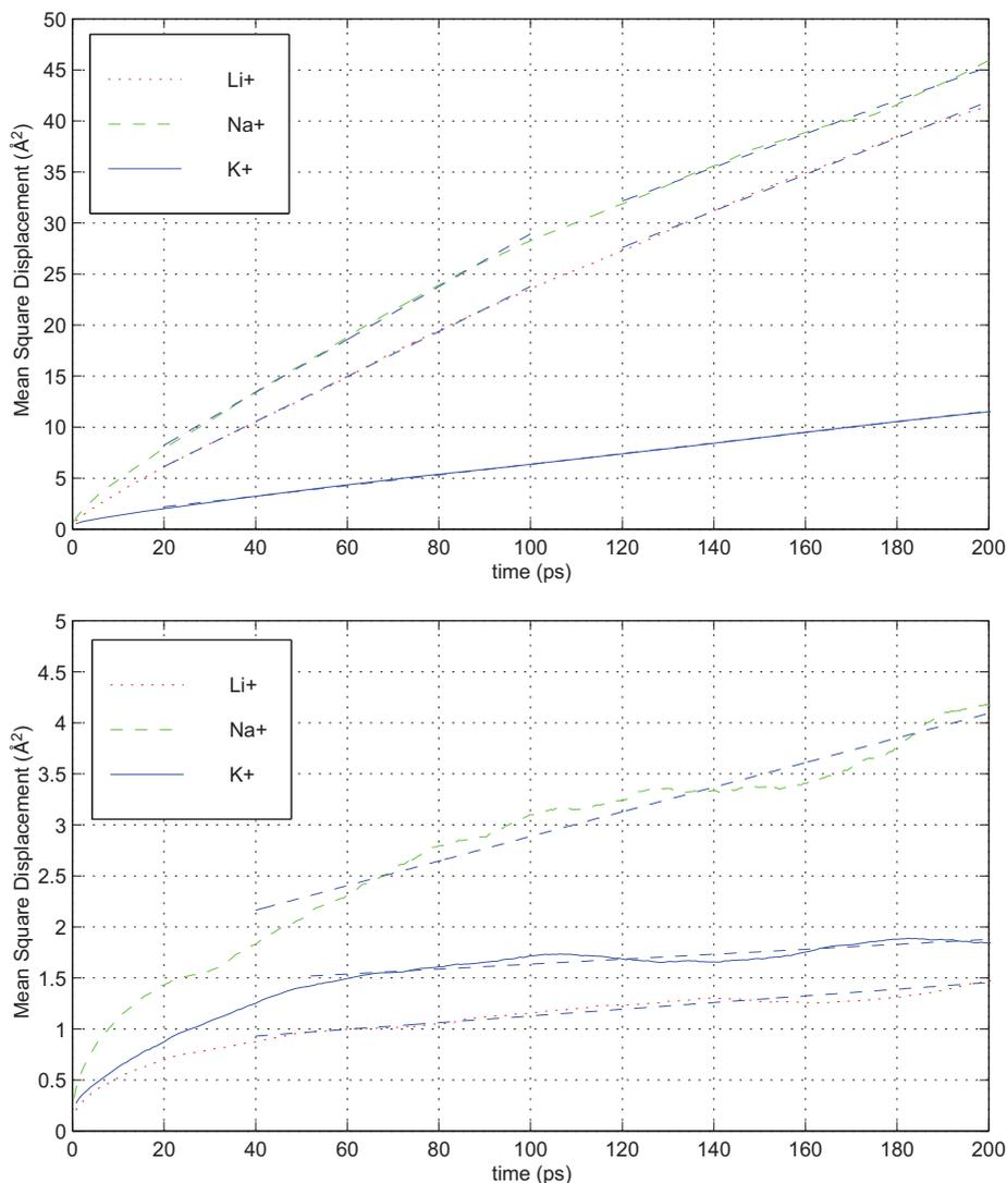
**Figure 6.** Mean-square displacement of water (upper) and cations (lower) in the interlayer space of Wyoming montmorillonite containing 32 water molecules.
