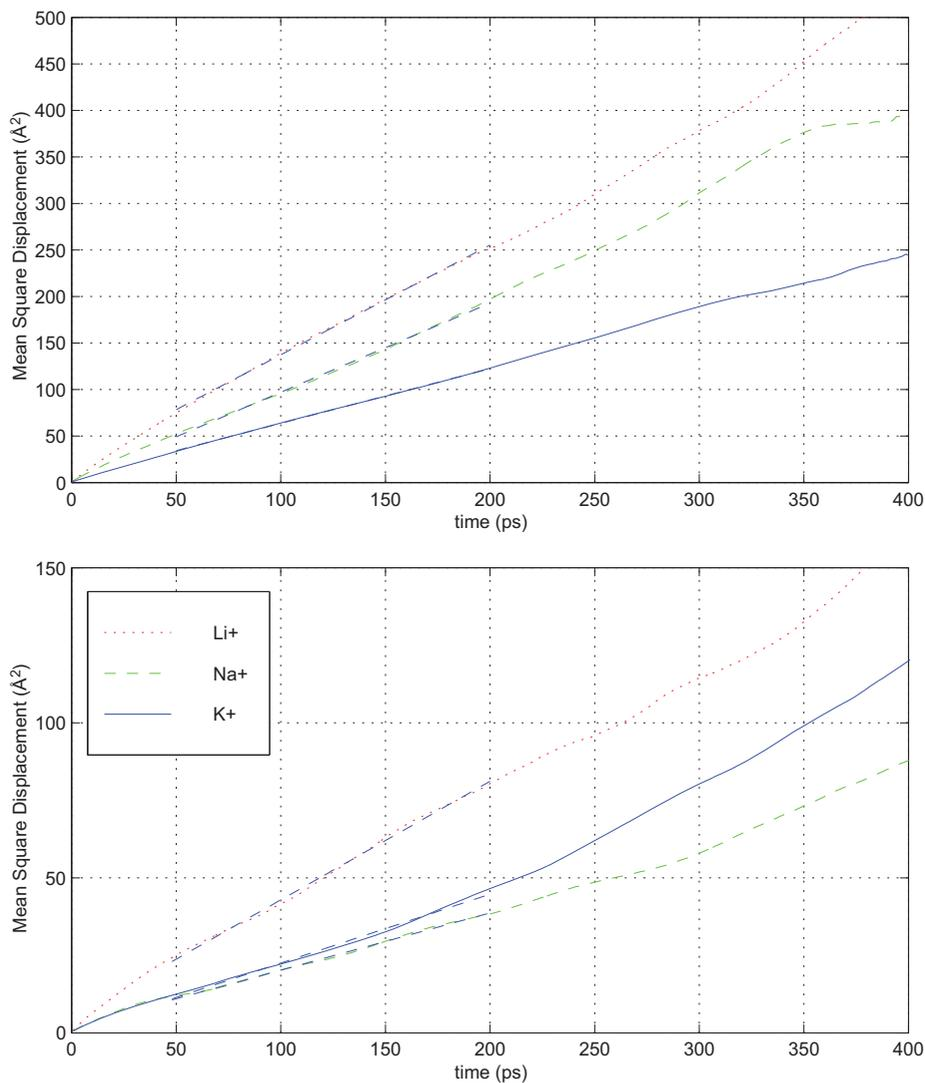
**Figure 8.** Mean-square displacement of water (upper) and cations (lower) in the interlayer space of Wyoming montmorillonite containing 96 water molecules.
