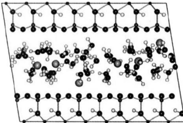
**Figure 5.** Unit-cell structure of hydrated montmorillonite showing equilibrium configuration of interlayer water molecules and  $\text{Na}^+$  ions (large gray spheres). Oxygen atoms are medium-sized black spheres, H atoms are small white spheres, and both Si and Al ions are small black spheres. Reprinted with the permission of the American Chemical Society from Boek *et al.* (1995).
