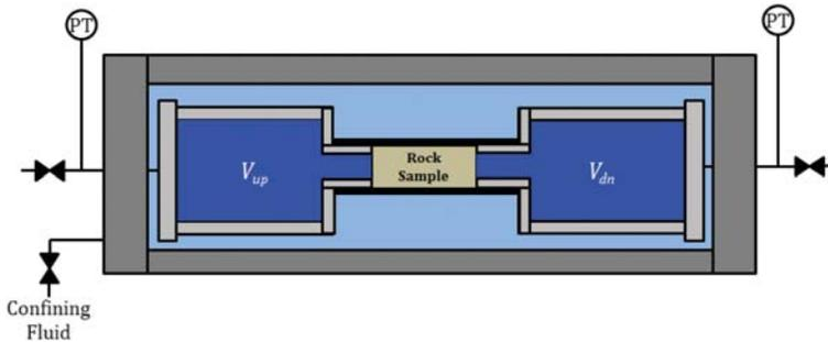
**Figure 1.** Simplified systemic diagram showing fluid reservoirs used for permeability determination experiments.
