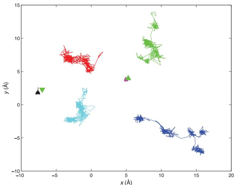
**Figure 9.** MD trajectories for Na<sup>+</sup> counterions in the single-layer hydrate.
