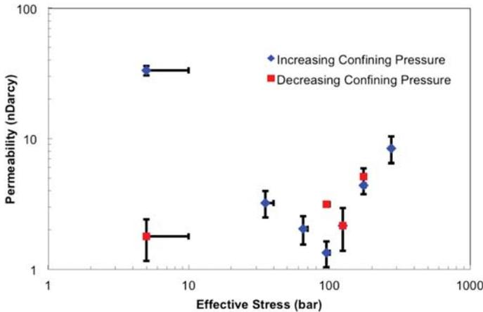
**Figure 2.** Permeability of the Hontomin shale sample for each effective pressure applied.
