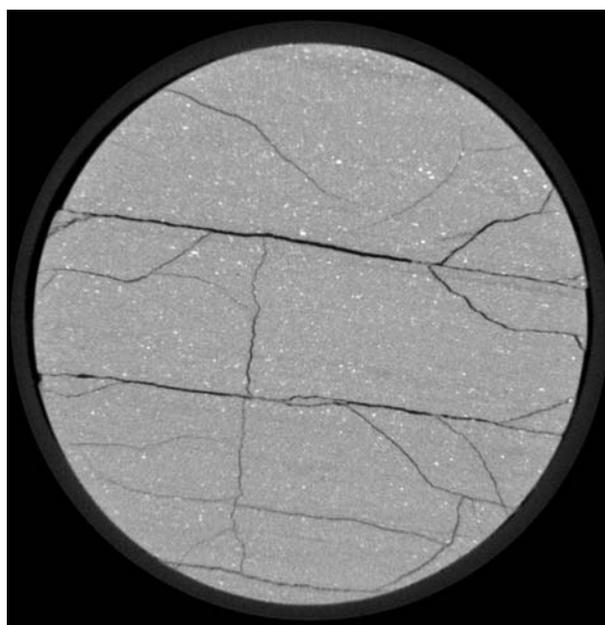
*Figure 4.* Tomogram of a shale sample after swelling from contact with untreated tap water.
