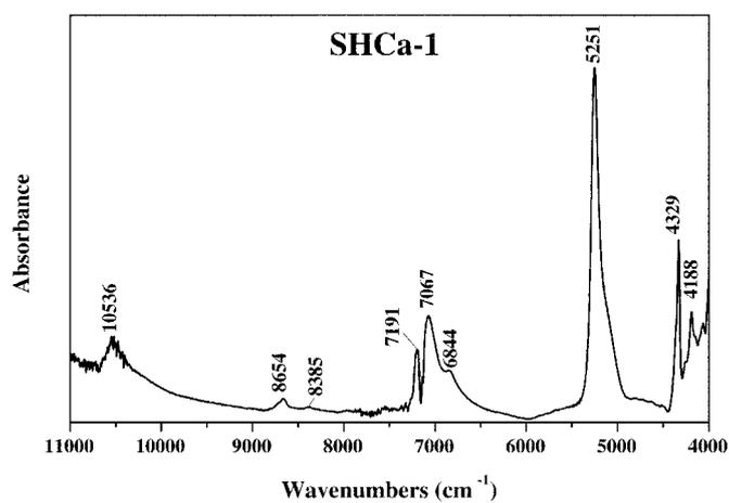
Figure 21. Diffuse-reflectance NIR spectrum of SHCa-1 (hectorite).
