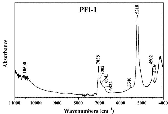
Figure 28. Diffuse-reflectance NIR spectrum of PFI-1 palygorskite.
