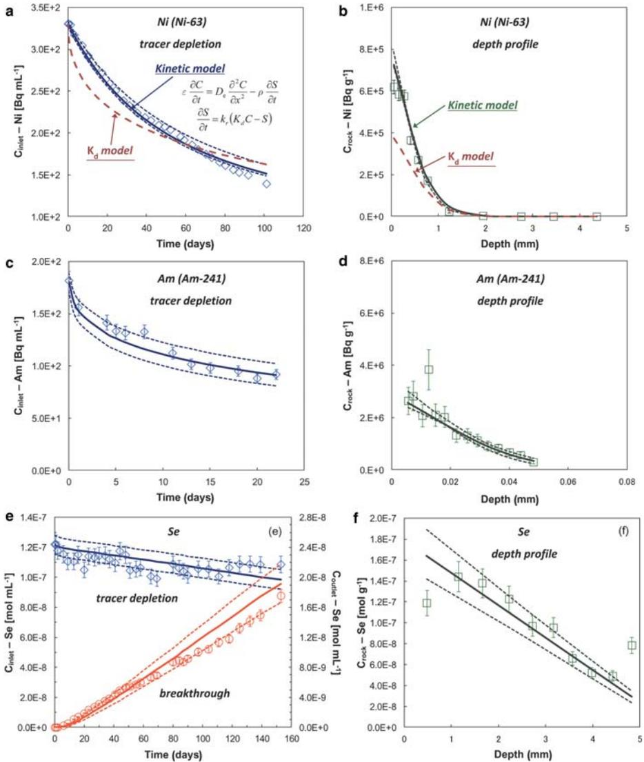
**Figure 1.** Typical results of through-diffusion experiments for: (a–b) Ni, (c–d) Am, and (e–f) Se(IV). Inlet depletion curves and outlet breakthrough curves are shown in parts a, c, and e, and depth profiles are shown in parts b, d, and f. The solid lines are best-fit curves obtained by simultaneous fitting of the diffusion equations assuming the  $K_d$  model (Am and Se) or the kinetics model (Ni). The dashed lines without remarks indicate ranges of uncertainty.
