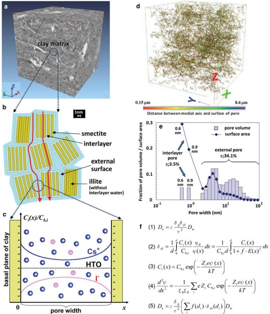
**Figure 3.** Conceptual images of diffusion model: (a,d) 3D images obtained by nano-focus X-ray CT and medial axis analysis; (b,c) simplified sketch of clay matrix and EDL in narrow pores; (e) pore-size distribution, and (f) equations of EDL diffusion model.
