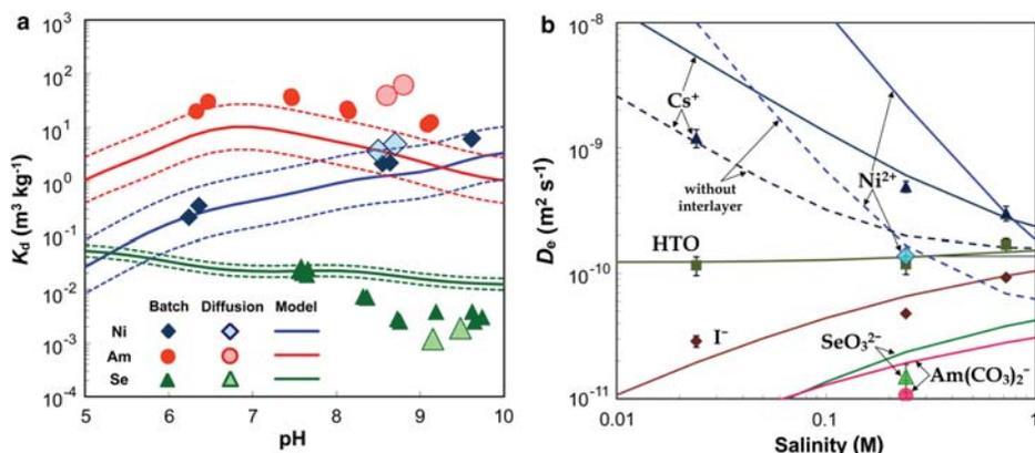
**Figure 2.** Comparison between measured and modeled results for Ni, Am, and Se: (a)  $K_d$  values and modeling result as a function of pH. The solid and dashed lines represent modeled results and uncertainty ranges, respectively. (b)  $D_e$  values and modeling result as a function of porewater salinity. The solid lines denote modeled results. The results for Cs, I, and HTO were taken from Tachi *et al.* (2011).
